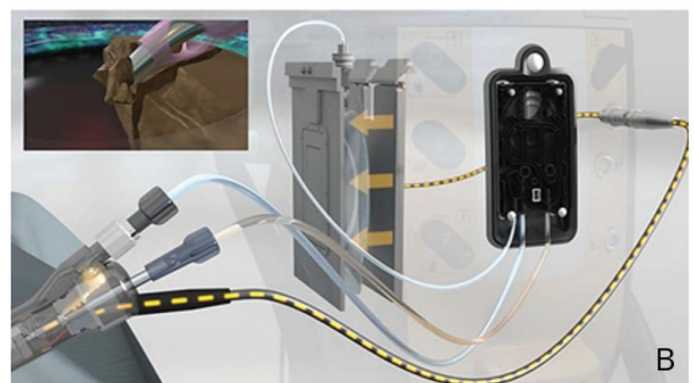
Figure 1. The Active Sentry® Handpiece features a built-in pressure sensor that reacts in real time (A). Active Sentry® communicates with hardware and software to compensate for changes in the anterior chamber (B). When occlusion happens, the system detects it and signals for a pressure adjustment to the BSS bag.
