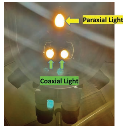
Figure 3. Illustration of paraxial and coaxial illumination in a surgical microscope. Paraxial lighting enhances the depth of field, and coaxial lighting is responsible for producing the red reflex.
