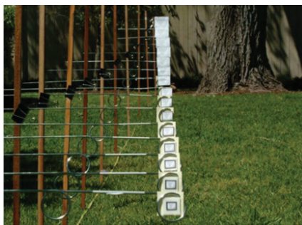
Figure 2. Photograph taken with a small aperture equivalent to that of an IOL in an eye with a 1.6-mm pupil and 3.00 D of continuous depth of focus.
