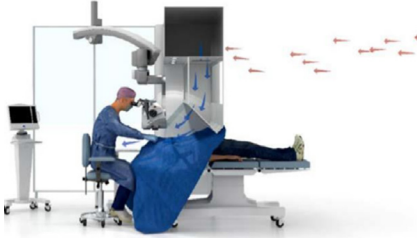
Figure 2. The SurgiCube allows an ultraclean surgical environment by supplying HEPA-filtered air to the OR using a unidirectional airflow technique.
