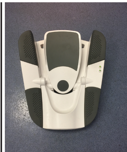
Figure 2. The Stellaris Elite has a dual-linear footpedal (left) with several interesting features, including the ability to uncouple control of the ultrasound power and fluidics (right).
