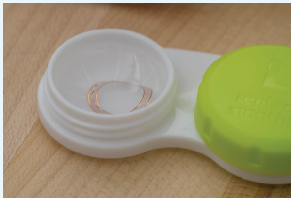
Figure 2. A contact lens modified with a coil to generate electromagnetic fields.
