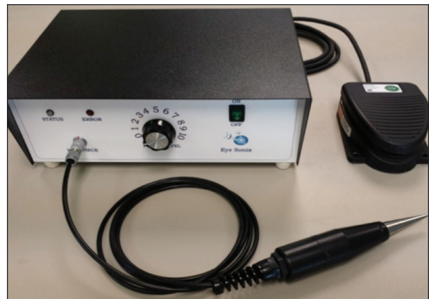
Figure 1. TUG is a portable, stand-alone, lightweight (5-lb) device that can be easily transported to satellite offices.
