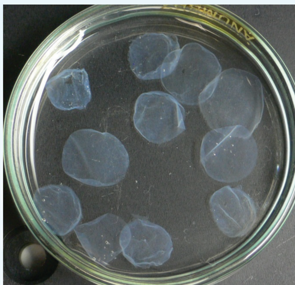
Figure 2. A demonstration of the femtosecond laser's ability to make thin sheets from a cornea (early development: porcine laminar sheets).
