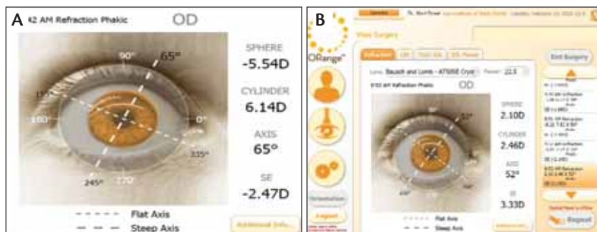
Figure 2. Screen images provided by ORange intraoperative aberrometer. The instrument detects significant astigmatism prior to suture adjustment (A). Intraoperative wavefront-guided suture adjustment reduced astigmatism considerably (B).
