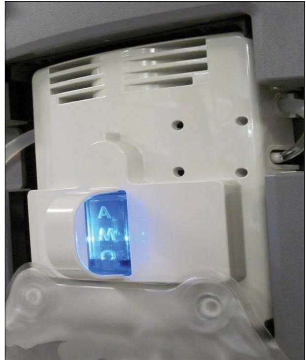
**Figure 3.** The Signature system's Venturi cassette uses a blue light beam to detect fluid levels instantaneously and turn on the venting pump as required.
