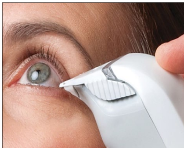
Figure 8. Trained office staff can perform the osmolality test. They lightly touch the tear meniscus at the lateral canthus in each eye with the handheld portable lab-on-a-chip reporter and then insert the device into a nearby digital reading station.
