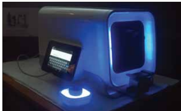
Figure 2. The MAPCATsf measures MPOD and provides an assessment of the lens and its functions.
