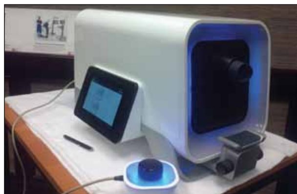
Figure 1. The MAPCATsf (Guardion Health Sciences) is a desktop heterochromatic flicker photometer.
