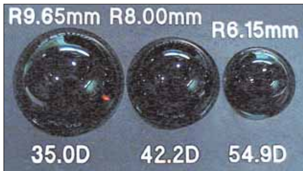
Figure 5. A standard set of calibration spheres (Carl Zeiss Meditec, Inc.). It is important to regularly check the calibration of all instruments used to measure the central corneal power.
