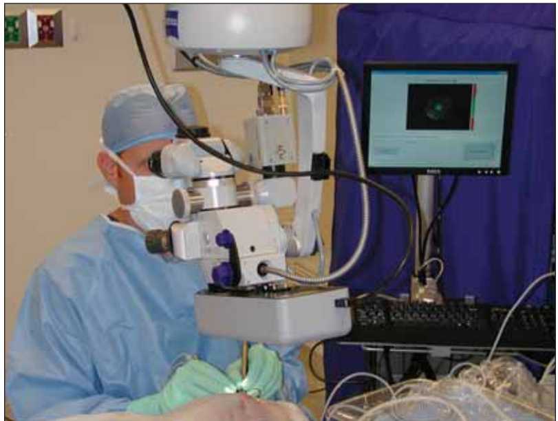
Figure 1. Dr. Weinstock uses the ORange intraoperative wavefront aberrometer. The device is attached to the bottom part of the microscope.
