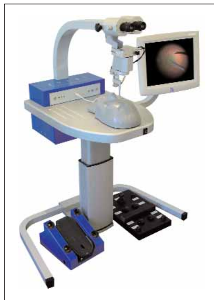
Figure 1. The Eyesi Ophthalmic Surgical Simulator is shown with the interchangeable cataract head software on its adjustable platform. The device's hardware includes control pedals for phacoemulsification/vitreotomy (left) and the surgical microscope's adjustment (right). The virtual operating microscope features a stereoscopic view of the surgical field.
