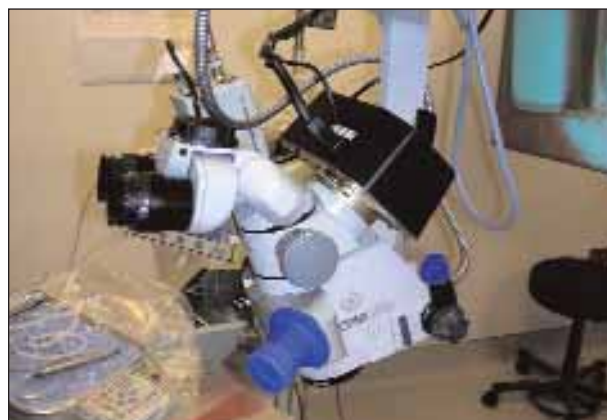
Figure 2. The image capture station sits behind the oculars of the microscope.
