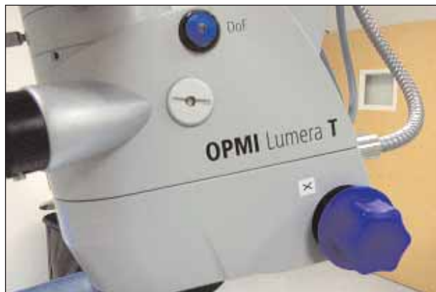
Figure 2. An autoclavable knob allows the surgeon to adjust the oblique illumination beam shutter.
