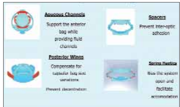
Figure 4. Features of the Synchrony dual-optic design are highlighted in red.
