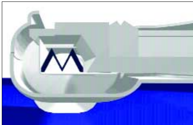
Figure 7. The Mport SI inserter (Bausch & Lomb) compresses the IOL into an "M" shape in preparation for insertion into the eye.
