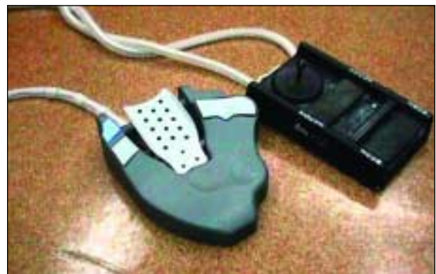
Figure 3. One-inch plastic tubing encases the wires of machines in the OR to keep the floor clear.
