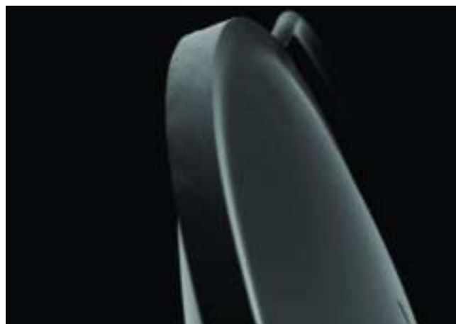
Figure 6. SEM photography (38X magnification) shows the truncated edge of the Soflex LI61SE IOL.
