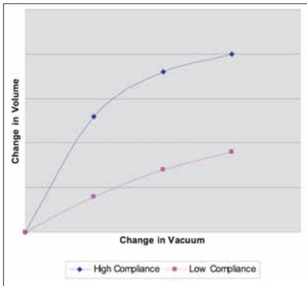
**Figure 1.** This graph demonstrates that low-compliance (rigid) systems are affected less by various vacuum pressures.
