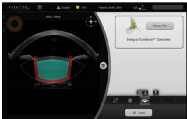
Figure 4. Powered by full-volume OCT imaging, the Catalys system's proprietary Integral Guidance system accurately maps ocular surfaces and designates safety zones to ensure laser pulses are delivered only where intended.
