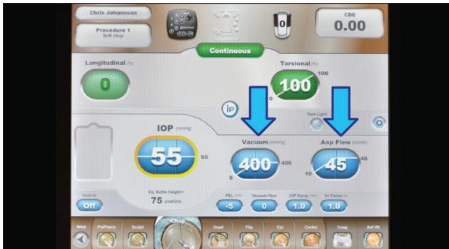
Figure 2. First, I set the vacuum at 400 mm Hg and the pump at 45 cc/min. Both are in linear mode, foot pedal position 2. With max vacuum set to 327, there is only 73 mm Hg of difference between the occluded and unoccluded states of the phaco tip.
