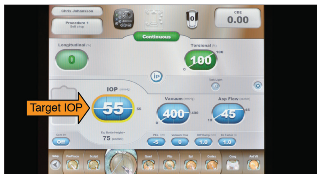
Figure 1. With a combination of pressure sensors and advanced calculations, the CENTURION Vision System is designed to maintain the target IOP that the surgeon sets at the beginning of surgery.
