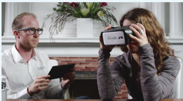
Figure 5. Users hold the EyeNetra device to perform self-refraction.
