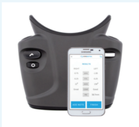
Figure 4. EyeNetra’s smartphone-based subjective autorefractor.
