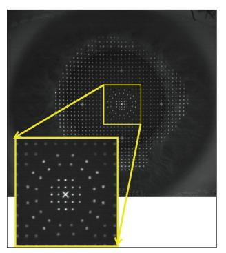
Figure. A full-gradient corneal topographer provides central corneal coverage. Central spots illuminate the corneal vertex area. The location of these spots does not depend on the distance to the eye or its position within the field of view.
